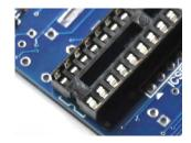
Flip the board over and solder one pin on each corner of both sockets. This makes it easy to reposition the sockets in case they aren't seated all the way down against the board; just reheat the corner pins and adjust the socket positions as necessary.
